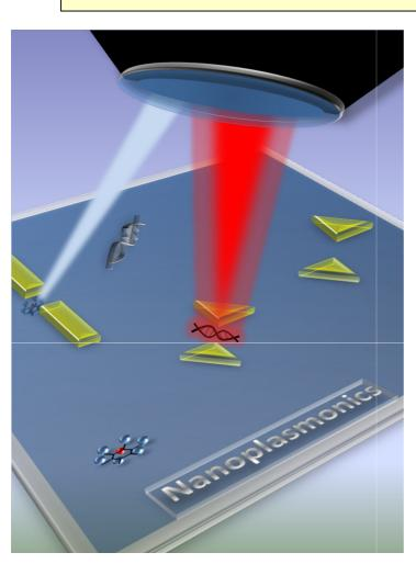
Controlling and guiding light has been one of science's most influential achievements. In particular, when light interacts with a metal nanoparticle, its conduction electrons can be driven by the incident electric field in collective oscillations known as localized surface plasmon resonances.
